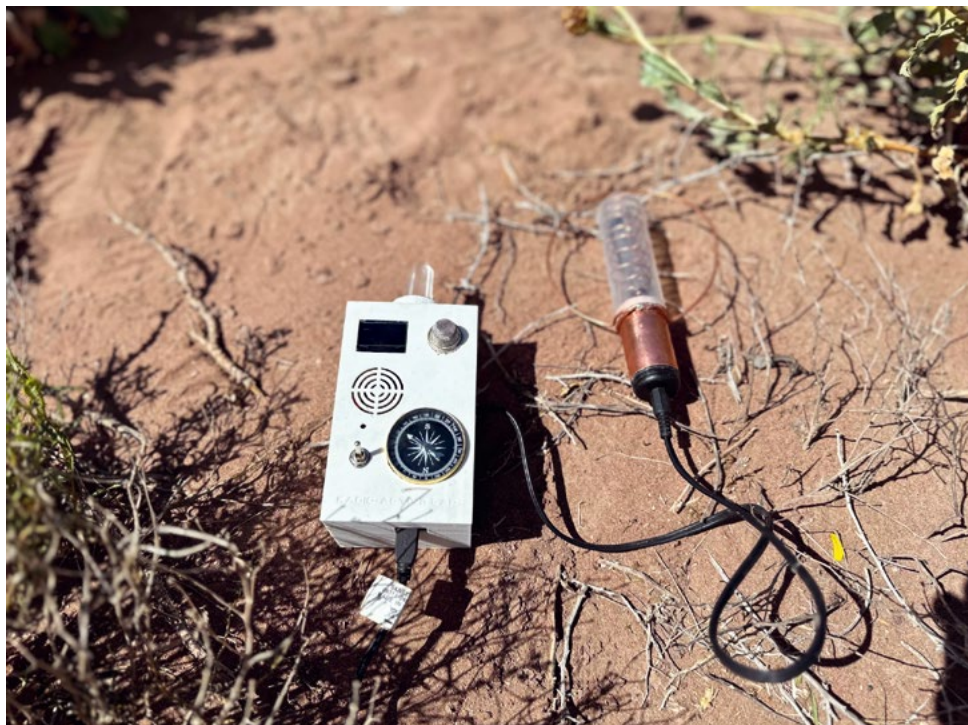
Fig 22. Open-source counter Geiger sensor. Image: Courtesy of the artist.
