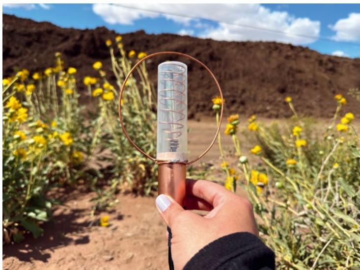
Fig 21. Radioactivity measurement exercises with DIY Geiger counter of cutting waste in open sky deposits, Añelo. Image: Courtesy of the artist.
